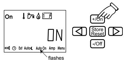
When you arrive at the vehicle, boat or building and AutoOn is activated, deactivate AutoOn to prevent the boiler from stopping after 24 hours (the boiler cannot be switched off when AutoOn is activated).
