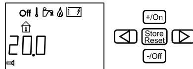
The pump is in automatic position. The lower menu row is not lit up.
