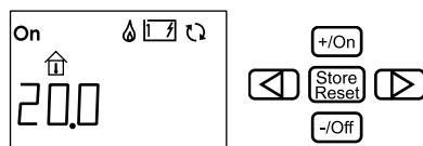
Start the on position by pressing any button. The background lighting comes on (blue light) and a function that can be set flashes. Select a function that can be set with the arrow keys. The settings are automatically saved.
